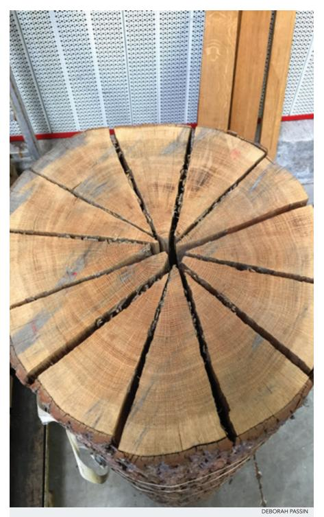
A log is split into 12 sections, called *quarters*, that will yield two to three staves each. This log represents a little less than one barrel.
