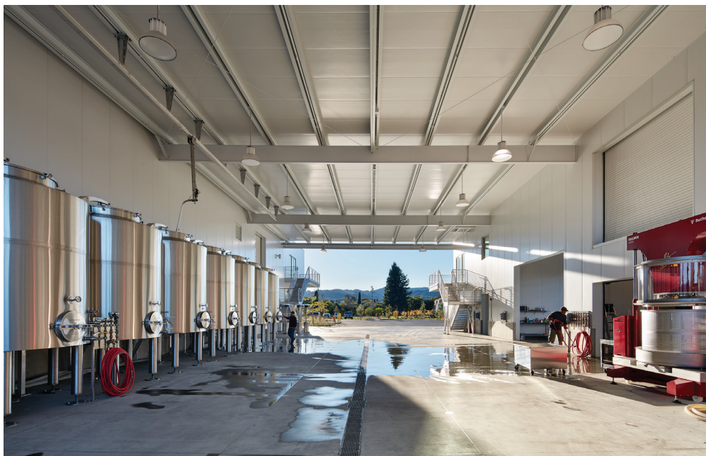
Tanks are equipped with TankNet data-logging and control system and pumps for automatic pumpovers.
