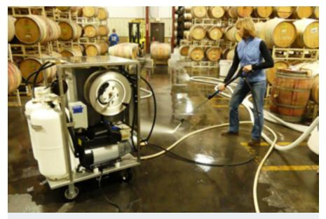
The all purpose HotCart from AaquaTools will power the impingment head inside your tank to disperse the the colloidal cleaner.
