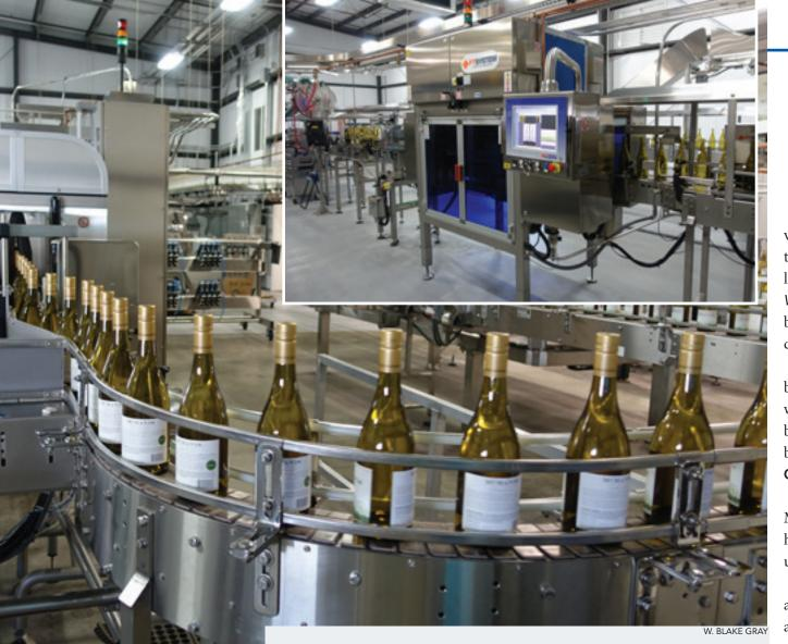
McManis installed a new bottling line that automatically eliminates defective or improperly filled bottles.
