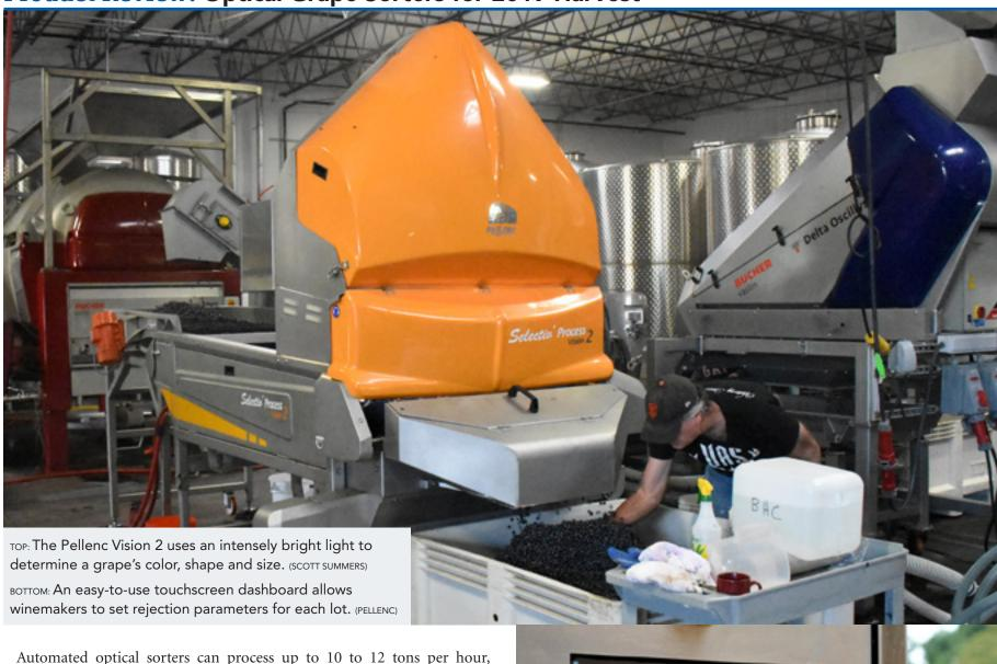
Automated optical sorters can process up to 10 to 12 tons per hour, depending on the model and incoming grape quality, driving sorting costs down to as little as \$20 per ton or \$0.30 per case. At that cost, a winery could sort most or all of its fruit, increasing the quality of every wine it makes.
