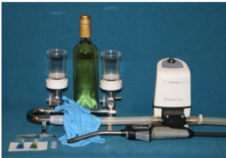
FIGURE 2. The parts needed for testing a bottled wine's microbiological integrity include a manifold supporting one to six Biosart Filter flasks, protective gloves, E-Jet vacuum pump, torch for sanitizing bottle top and prepared media ampules.
