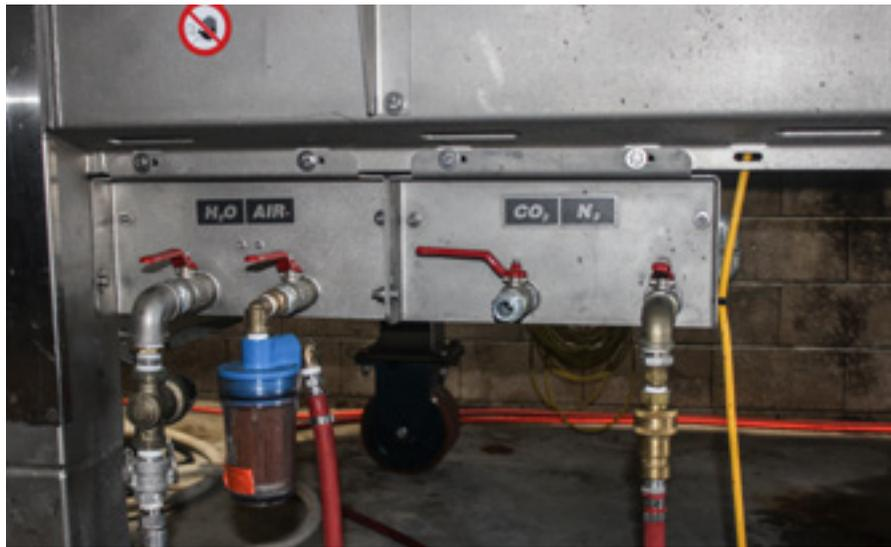
The Diemme Neutral 2 uses a fresh volume of nitrogen or carbon dioxide each time the press is deflated.
