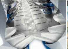
The proven NORIA system, with its polyurethane baskets, ensures the most gentle treatment of the vines and harvested crop, without ground losses.
