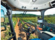
The BRAUD harvester cab is fully suspended and sound-proofed for a smoother, more comfortable ride. The pressurized cabs with heat and air-conditioning offer optimum comfort and protection during harvest, spraying and other operations.
