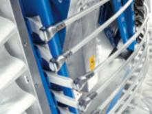
The BRAUD SDC system is recognized as the best picking system in the industry. Each shaking rod is independently hinged for perfect control of the shaking action, with maximum flexibility for gentle picking.
