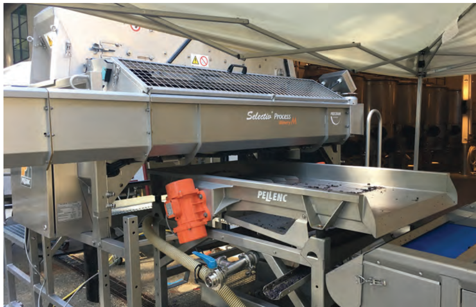
A Pellenc Selectiv Process destemmer and optical-sorting machine get red grapes ready for fermentation.
