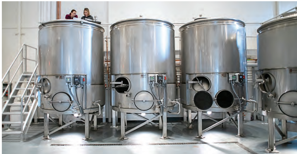
20 fermentation tanks from Westec are jacketed, insulated and equipped with centrifugal pumps from Process Engineers.
