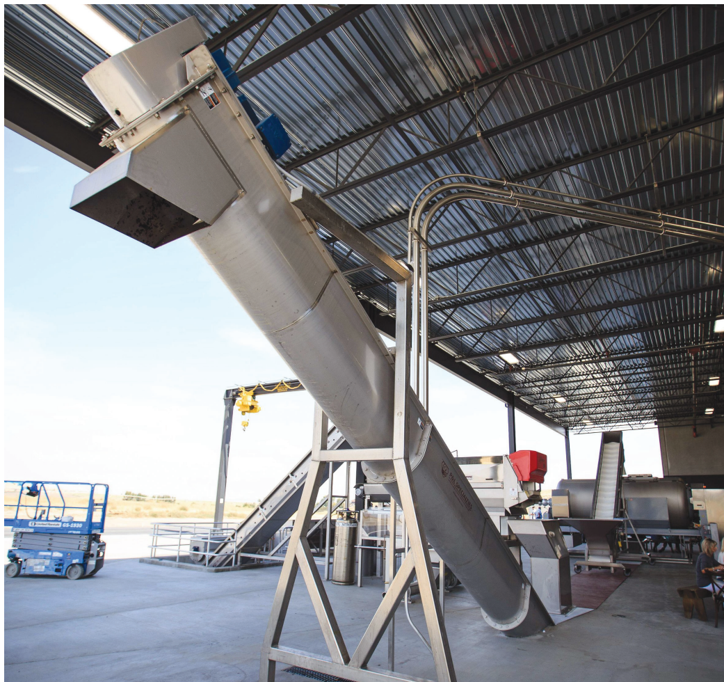
Several configurations of the Diemme Kappa 50 destemmer-crusher give Double Canyon maximum flexibility over incoming fruit.
