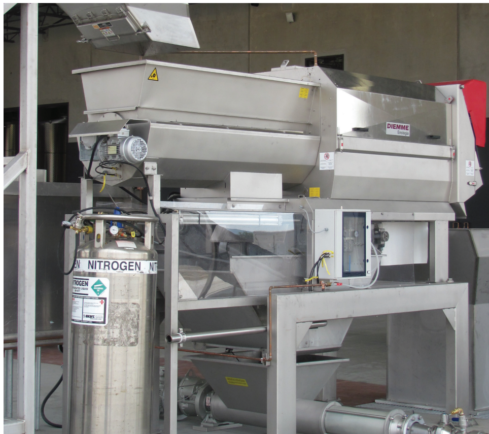
Nitrogen gas rather than water pushes fruit and must into tanks, saving water and preventing dilution.
