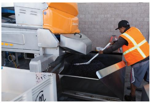
After destemming and sorting, the berries are collected into stainless steel sumps that are dumped into open-top tanks.
